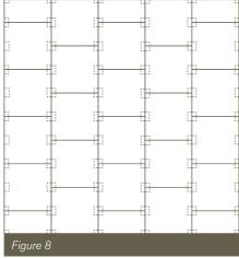
Lay anchor rows, placing a TacTiles connector at every joint. Install carpet tile using a step method in all quadrants, placing a TacTiles connector at every joint.
