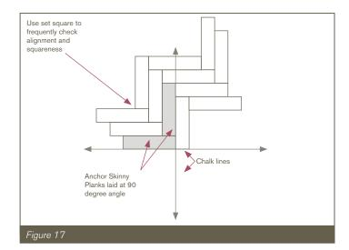
Type B is more complex and requires additional, diagonal working lines. Establish the centre focal point for the desired pattern and snap the centre and base chalk lines as described in section 3.2. Use the set square to check the chalk lines are perpendicular.
